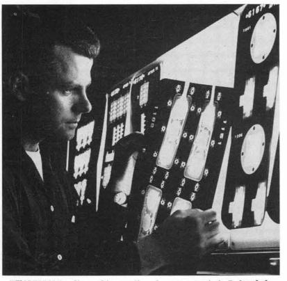
**EXAMINING** radiographic negative of a component, A. J. Arenholz (7233-2) uses an array of fluorescent panels as a light source.
